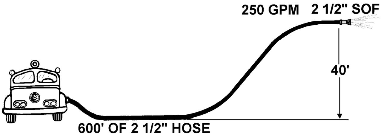
➤ **Step One:** Flow = 250 gpm
