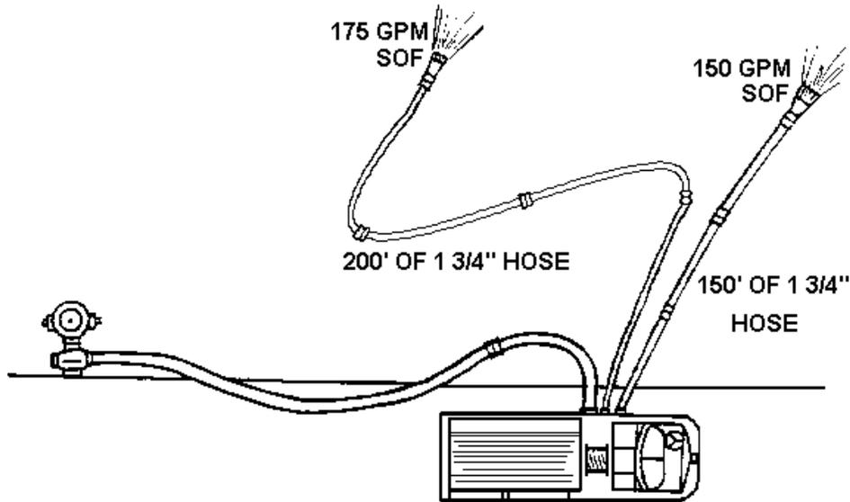
➤ **Step One:** EF = Factor x gpm
