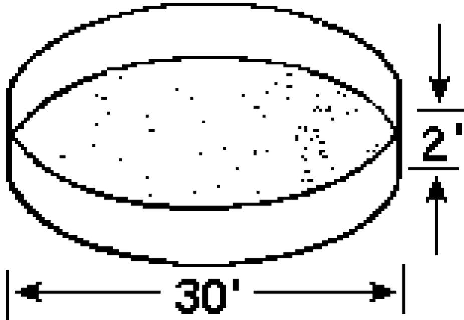
Example: Determine the weight of water in a cylindrical tank 30' in diameter and 2' deep:
