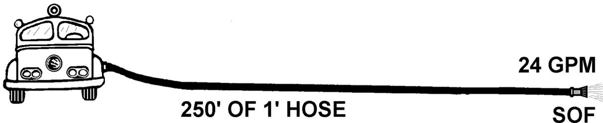
➤ **Step One:** Flow = 24 gpm
