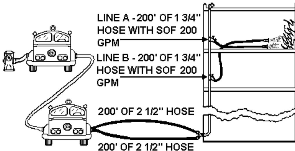
ALLOW 25 PSI LOSS FOR STANDPIPE SYSTEMS (SL) REGARDLESS OF SIZE. \*
