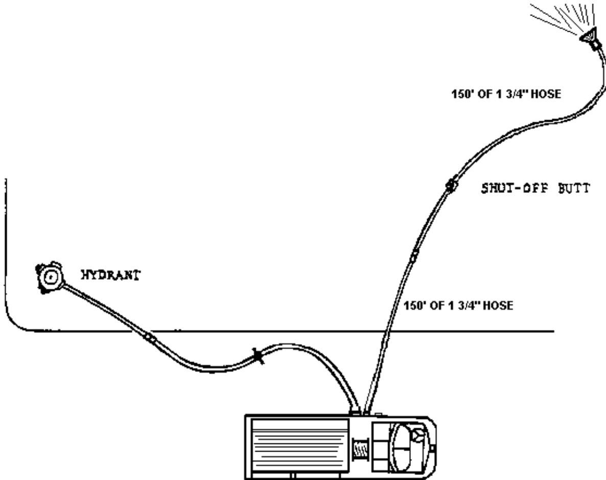
➤ **Step One:** Flow = **95 gpm**
