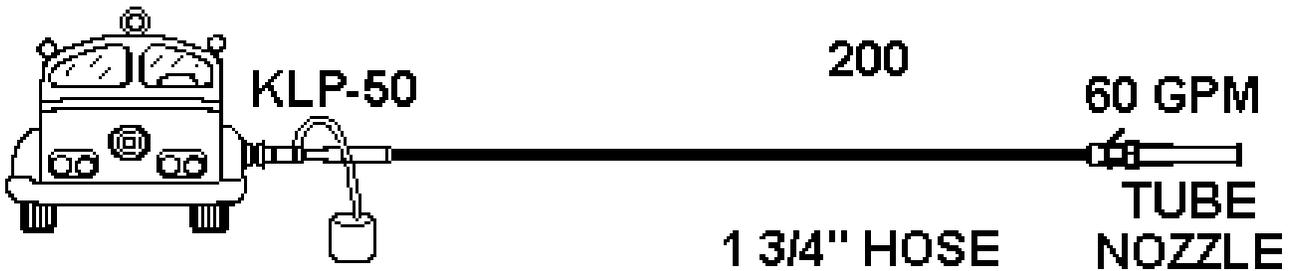
**NOTE: NO HYDRAULIC CALCULATIONS FOR ANY 1 3/4" FOAM LAY UP TO 600 FEET.**
