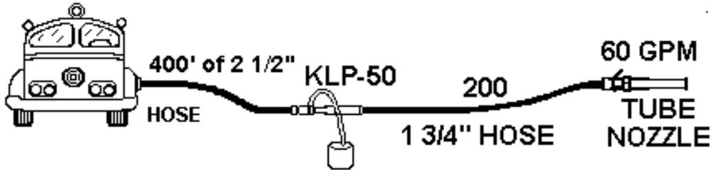
➤ **Step One:** Flow = 60 gpm
