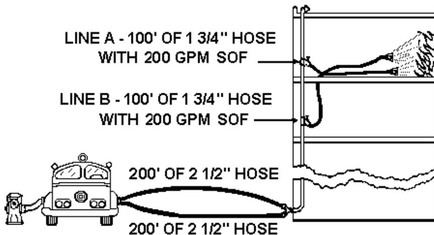
ALLOW 25 PSI LOSS FOR STANDPIPE SYSTEMS (SL) REGARDLESS OF SIZE. \*
