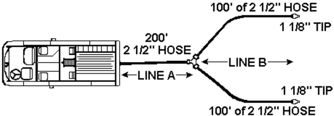
TO DETERMINE THE FLOW IN THE SUPPLY LINE, COMBINE NOZZLE FLOWS.\*
