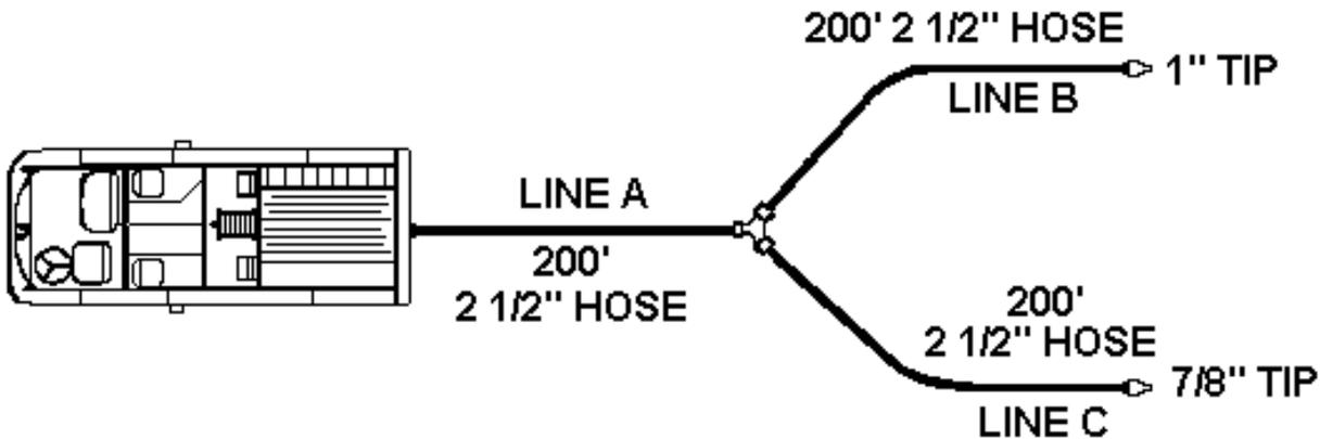
TO DETERMINE GPM FLOW, AVERAGE THE FLOWS FROM THE NOZZLES. \*
