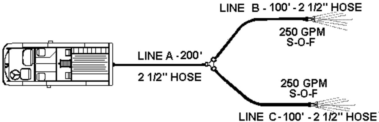
TO DETERMINE THE FLOW IN THE SUPPLY LINE, COMBINE NOZZLE FLOWS.\*
