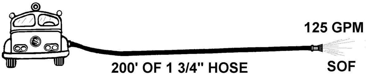
➤ **Step One:** Flow = 125 gpm
