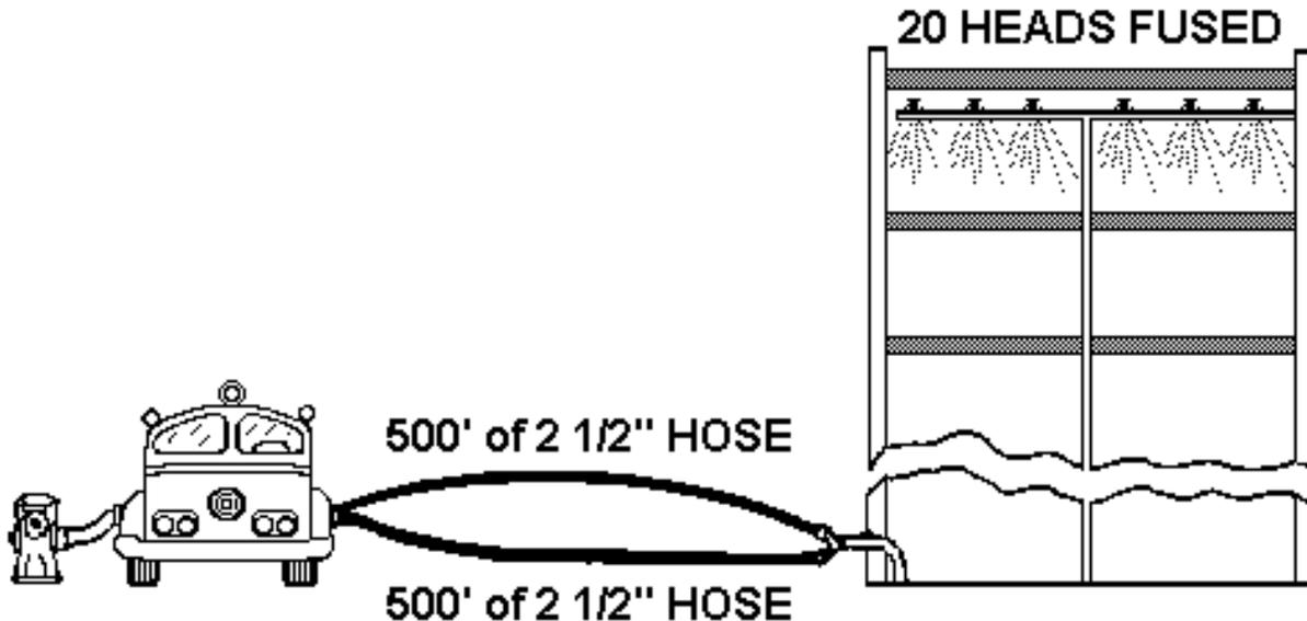
IN RAPID METHOD HYDRAULICS ALLOW 30 GPM PER SPRINKLER HEAD.\*
