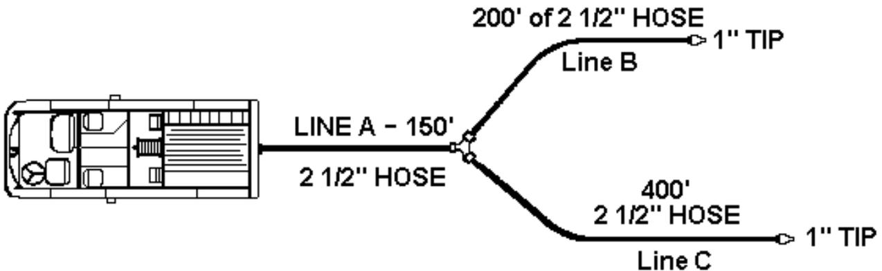
TO DETERMINE L, AVERAGE LENGTHS OF WYED LINES. \* When the average comes out to a 1/4 or 3/4 length, round off to the nearest 1/2 or full length respectively.
