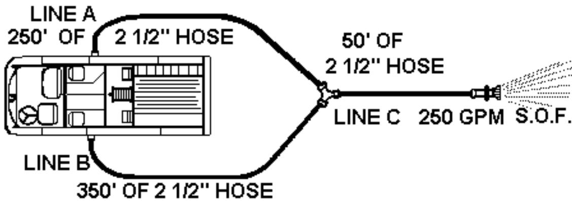
➤ **Step One:** Flow = 250 gpm
