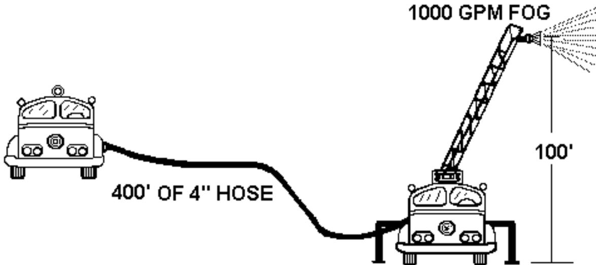
➤ **Step One:** Flow = **1000** gpm
